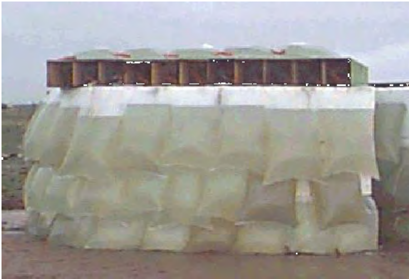
Water held in plastic bags as a bomb shelter to mitigate blast effects
